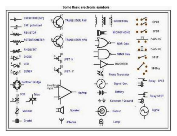
• Provides a short-cut method of drawing/expressing electronics circuits
